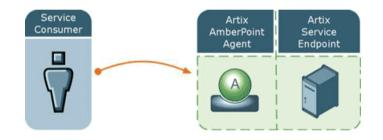
An Artix interceptor is deployed on the dispatch path of all messages exchanged between Artix service endpoints and consumers. It may be deployed in the same process as the consumer and/or the endpoint, or as an intermediary between the consumer and service.
