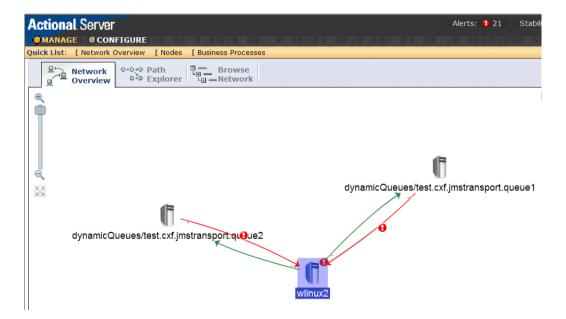
The **Network Overview** screen provides a high-level overview of the nodes in your network, and displays details such as the flow of calls and alarms between them.
