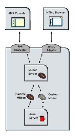
The custom MBeans shown in Figure 4 are optional components that can be implemented as required (for details, see Chapter 3).
