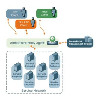
Because all messages are routed through the AmberPoint Proxy Agent, the additional network hops may impact on performance. In addition, the proxy involves the risk of a single point of failure.
