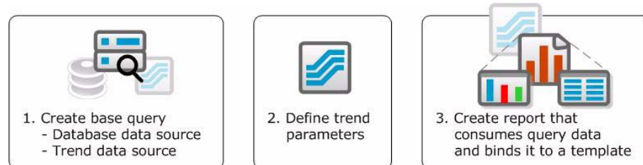
Figure 8-5 The anatomy of a trend. To develop a trend, first create a query that defines the data you are interested in. Next, define the trend time period and other parameters. Finally, you can use the resulting trend data in a report.
