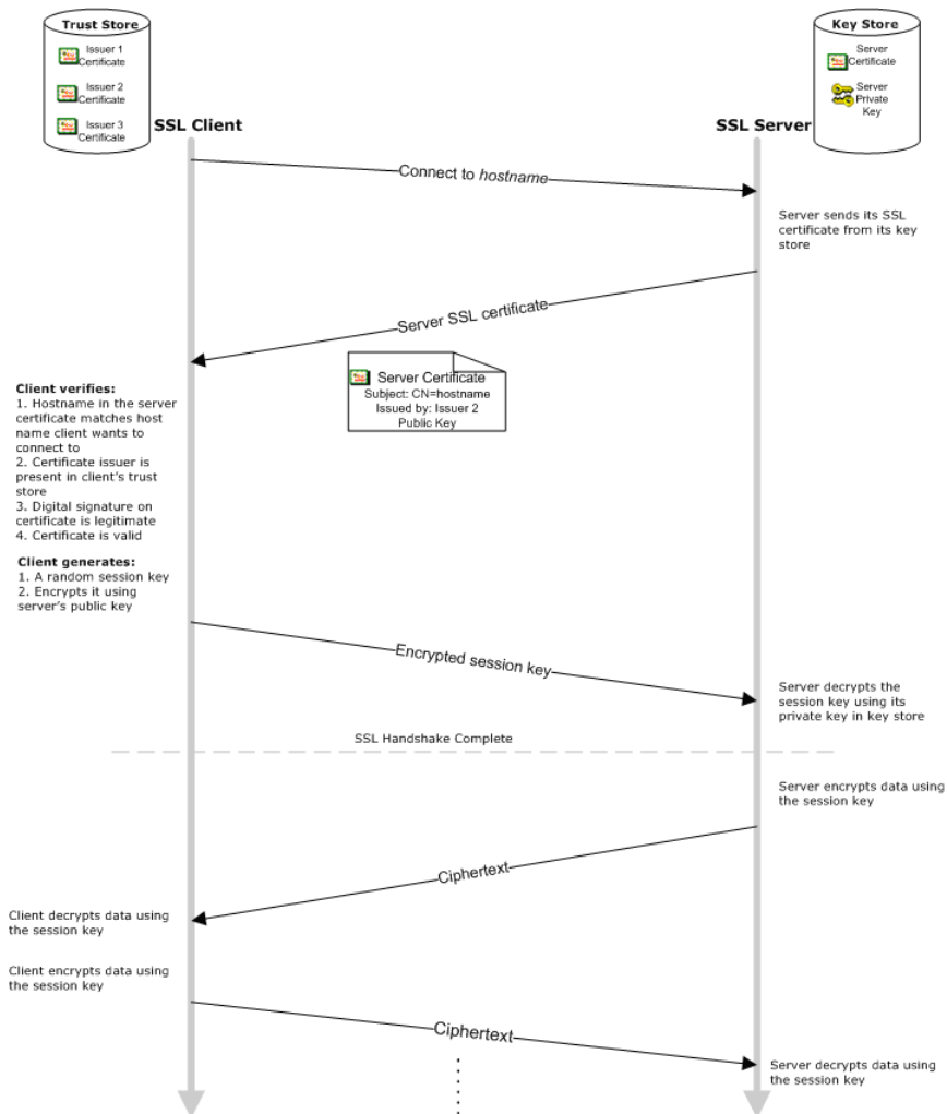
Figure 2-1 SSL handshake between an SSL server and client
