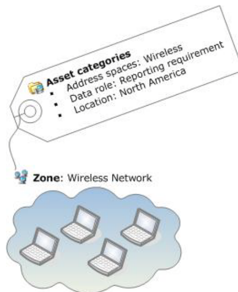
Figure 11-15 Categories assigned to zones. For situations where assets are not fixed, such as a wireless or VPN network, you can assign categories to a zone.
