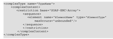
When using this syntax, the element's maxOccurs attribute must always be set to unbounded.
