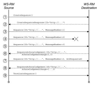
Figure 19: Sample WS-RM Message Exchange Pattern
