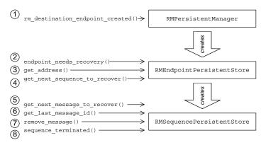
Figure 24: Overview of Recovering a Destination Endpoint
