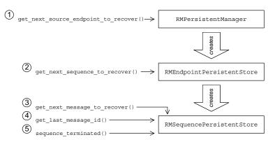
Figure 22: Overview of Recovering a Source Endpoint
