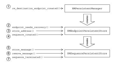
Figure 23: Overview of Persisting a Destination Endpoint
