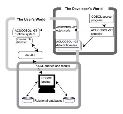
After your ACUCOBOL-GT data dictionaries have been generated, you can switch to a different RDBMS simply by linking in a different Acu4GL module and setting **DEFAULT\_HOST** to point to the new RDBMS. No recompiling is necessary.
