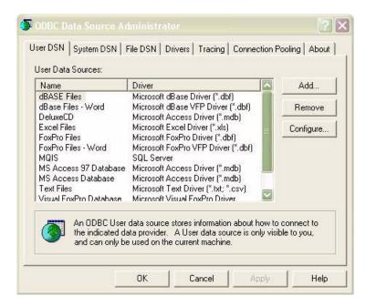
3. Double-click on the data source you plan to use to access a setup dialog. A subsequent window lets you add a description of the data source and allows you to supply other information the driver requires.
