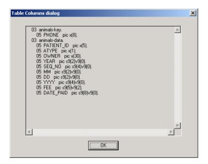
Note that PHONE appears first, even though it is not the first column in the table. That is because PHONE was defined as the table's key, so **acu4glfd** treats it as a unique index, moving it to the top of the list of columns.
