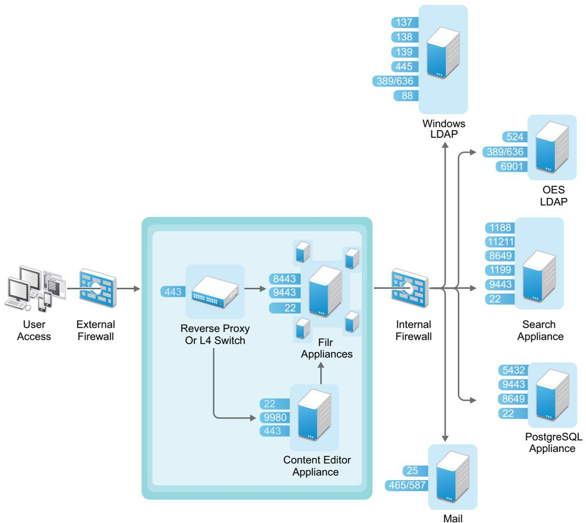
Only traffic destined to the DMZ is allowed through the front-end firewall, and only traffic from the DMZ to the internal network is allowed through the back-end firewall.
