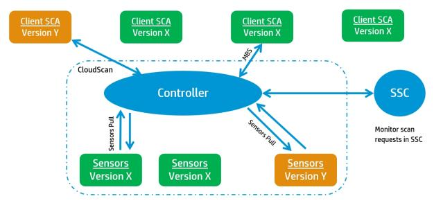
Sensor (virtual) machines - autonomous, dedicated to run SCA scans. Manage infrastructure using standard IT remote management tools
