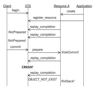
Figure 14: Use of the replay\_completion() operation
