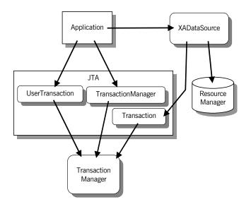
Figure 4: Application and Resource Manager Interaction using JTA
