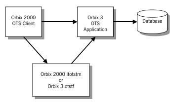
Figure 16: Interoperability with Orbix 3 OTS Applications
