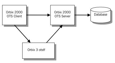
Figure 17: Using and alternative OTS Implementation
