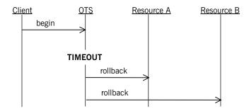
Figure 7: Rollback after a timeout
