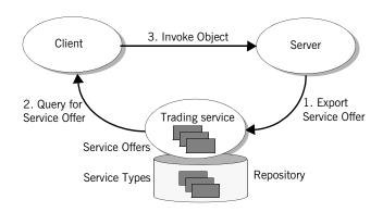
Figure 1: Typical trading service process
