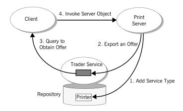
Figure 3: Typical Interactions with the trader
