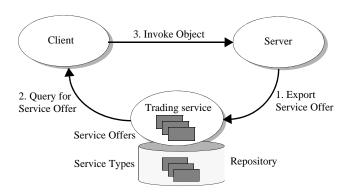
Figure 1: Typical trading service process
