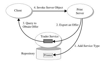
Figure 3: Typical Interactions with the trader
