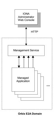
Figure 7 shows how IONA Administrator interacts with managed applications to provide management capabilities.
